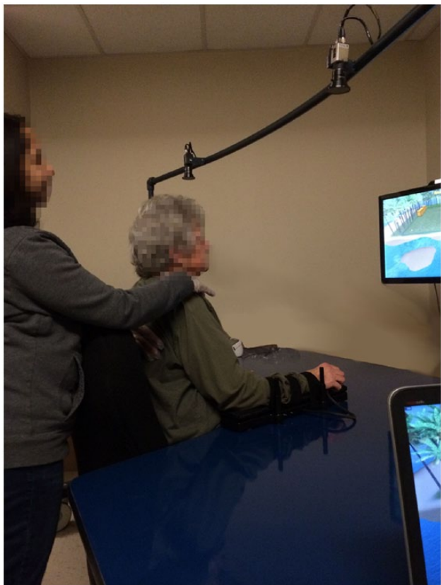
Figure 1. Subject training on BrightArm Duo Rehabilitation System when work surface was tilted upwards. Subject uses left and right arm supports to control virtual paddles in the Breakout 3D game. ©Bright Cloud International Corp. Reprinted with permission.
